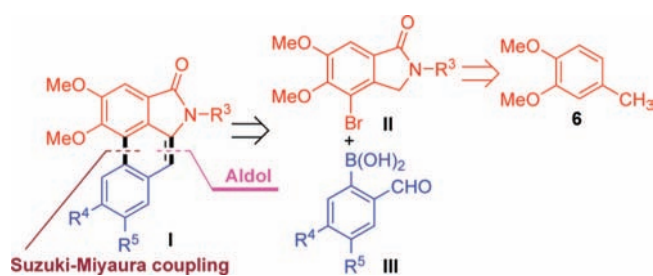
Scheme 1. Construction of a Phenanthrene Lactam via Suzuki–Miyaura Coupling/Aldol Condensation Cascade Reaction
